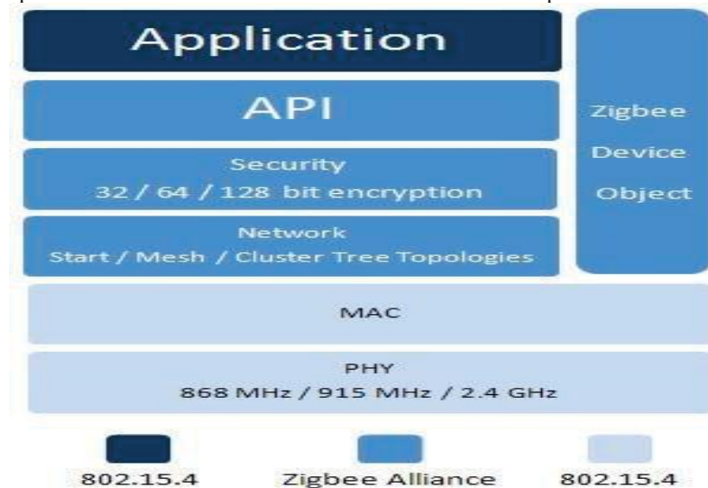
Fig. 2 Zigbee communication layers [7].
