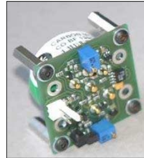
Figure 3. Photograph of an Alphasense signal conditioning module for one of their carbon monoxide sensors.
