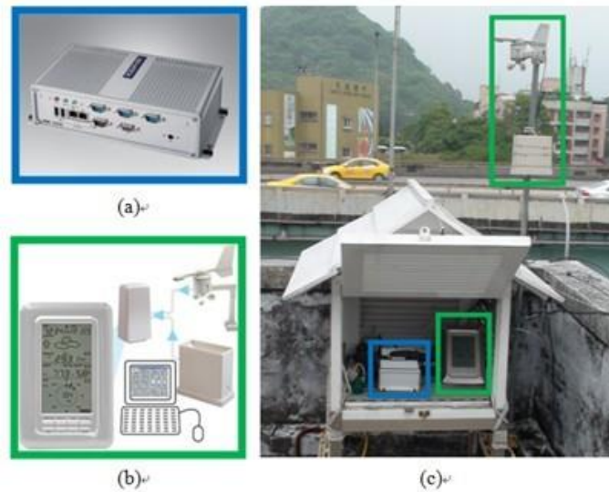
Figure 13. The proposed gateway (a) ARK-3360L Industrial PC [18]; (b) Weather station module WS-2316; (c) The actual settings of the gateway
